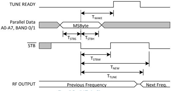
Figure 7. Parallel Timing Diagram
