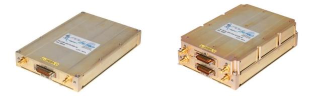
Out of band RF power handling refers to signals that are at least twenty percent (20%) removed from the tuned center frequency and is frequency dependent: 5W signals applied between 30 and 75 MHz, 8W from 75 to 175 MHz, and 10 W from 175 to 520 MHz. © Pole/Zero 2017
